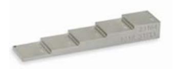
Thickness and linearity calibration. This 5-Step block is the metric "A" version.
