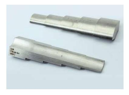
Thickness and linearity calibration. This 5-Step block is the metric "A" version.
