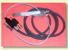
probe is up to the task. The sensitive element is embedded in stainless steel and the air cooling system allows the probe to be kept at ambient temperature without placing any thermal compromise on the welding operation. The extension cable is useful for large diameter pipes or if Zeromag is to be operated away from the job. Additional extension cables can be added for larger distances.
