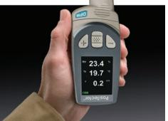
**Flip Display** enables right-side-up viewing in any position. PosiTector DPM A shown.
