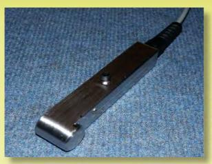
The MF500M provides an indication of the amount of magnetite within steam tubes. It assumes that the containing tube is essentially non-magnetic made usually of stainless steel. The magnetite is magnetic with magnetic properties similar to iron. This provides a route to measure the levels of
