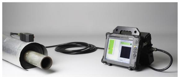
PECT instrument, showing data acquisition tablet computer that is permanently attached to a data acquisition and pulse generating unit. Instrument operation is from a touch screen.
