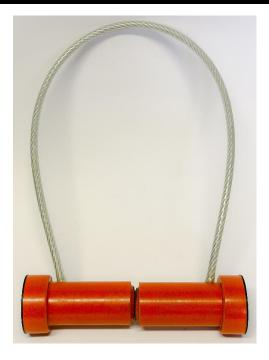
All Cable Type Permanent Yokes, when not in use, should be left with the Pole Pieces together. With the WM-5 and WM-5LT, this means simply allowing the Pole Pieces to come together. The WM-5C has more than sufficient length to bring the face of the Pole Pieces together.
