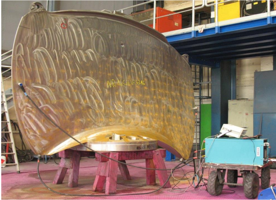
Fig. 6. MT-testing of a blade for a hydroelectric power plant (W= 4.5 m; H= 3.0 m) with direct current flow
