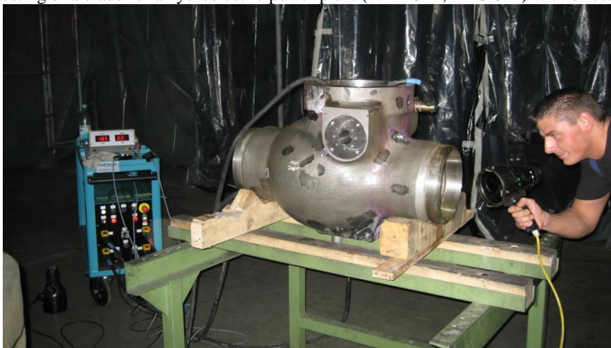
Fig. 7. MT-testing of a safety valve with direct current flow
