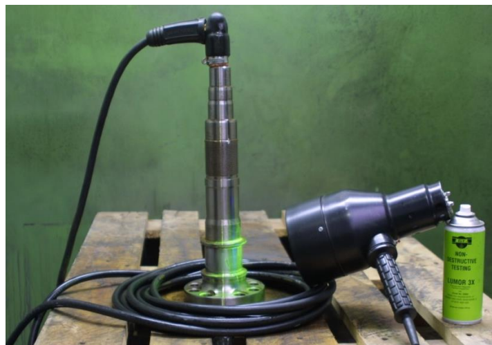
Fig. 8. Combined MT-testing of a blade shaft for an industrial fan for a power plant
