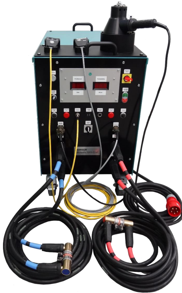
Fig. 14. Hirsch Unit, type Multipuls-1003-E2-2 (current peak= 30,000 A) with an increased duty cycle and integrated measuring device for impulse field, residual field and DC current measurement, type Multipuls-1003-M
