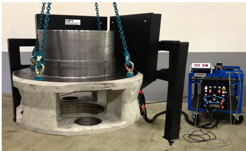
Fig. 11. Non-contact MT-testing and demagnetization of a planet-wheel carrier with two coils and the Hirsch Unit, type Multipuls-1003-E2-1 (30,000 A)
