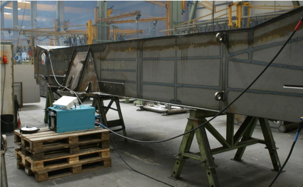
Fig. 4. MT-testing and demagnetization of a center beam of an automobile crane (9 m length)
