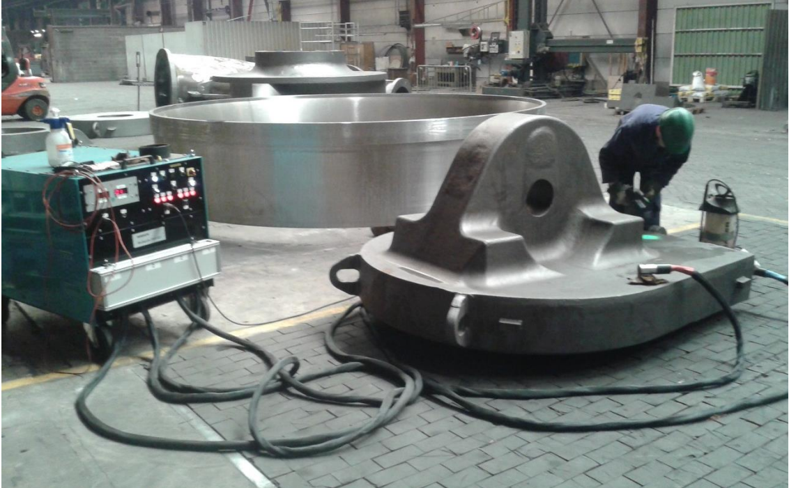
Fig. 17. Mt-testing of a casted component with direct current flow using 3 DC Pulse Technology
