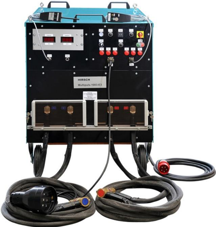
Fig. 16. Hirsch Unit, type Multipuls-1003-E3 (current peak= 3 \times 30,000 A) based on the new 3 DC Pulse Technology for MT-testing of large metal components with rough surfaces
