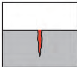
The surface is wiped clean but dry penetrant remains in crack.
