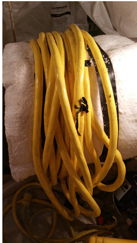
Demagnetizing cable wrapped on a fire blanket for protection from pre-heat
