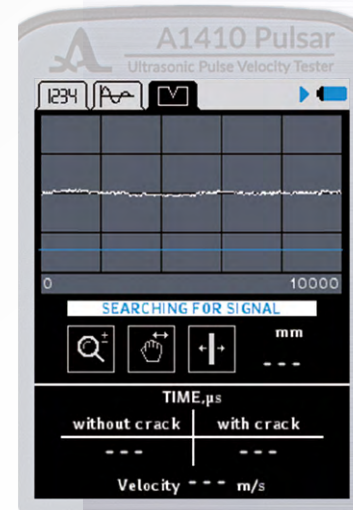
Figure 38: Crack Sizing Mode screen before calibration
