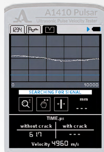
Figure 42: Device ready for crack measurements
