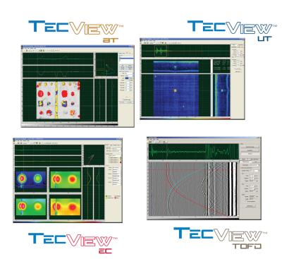
**TecView™** consists of a suite of software packages that comprises Ultrasonic, Eddy Current, Pulsed Eddy Current and Time-Of-Flight-Diffraction technologies. Combining the best of Windows operating systems and graphical user interface, TecView™ makes the NDT process simple and rapid. The software aids the user to setup the inspection parameters and it incorporates different modules including Data Acquisition and Management, Robotic control, Imaging as well as Data Analysis and Interpretation.
