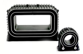
Annis demagnetizing coils have custom finished cast aluminum housings are designed for surface or bench mounting and have a 'ribbed' outer periphery to enhance convective heat transfer. These demagnetizers have field strengths that range from 210 to 1400 gauss and are designed for either continuous [C] or intermittent (I) operation in a dry environment.
