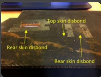
Figure 3: Thin CFRP honeycomb sample with rear surface disbonds.
