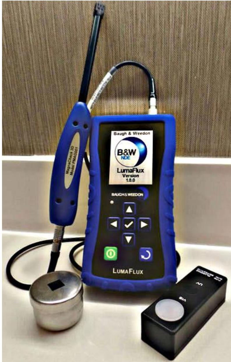
The LumaFlux combines all the established functions of the LumaCheck Dual UV / White Light Meter and the unique benefits of the MagnaCheck 3D Tangential Field Strength Meter in one rugged instrumentation package. With the easy “Swap & Go” system to change sensors, the LumaFlux automatically recognizes the Sensor that is connected and operates in the selected mode until the sensors are swapped again.
