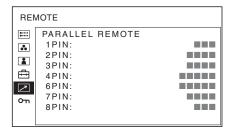
You can assign various functions to 1 to 4 pins and 6 to 8 pins. The following lists the functions you can assign to the pins.
