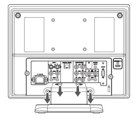
**2** Attach the mounting bracket, then attach the unit to the rack.
