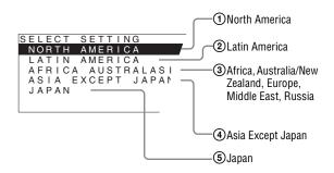
Press the ↑ or ↓ button to select the area where you intend to use the unit and press the → or ENTER button.
