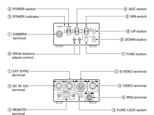
① CAMERA terminal Connects to the camera head.
