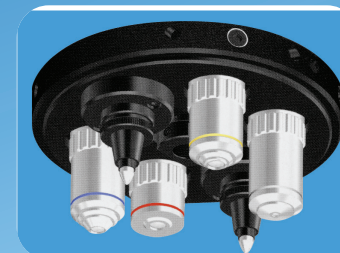
Optional dual indenter auto-turret allowing up to four objectives. (Available on CM-802 series only.)
