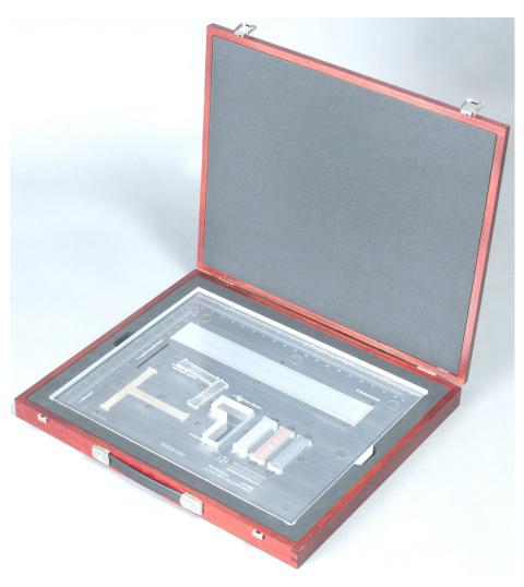
CR Phantom for Qualification of CR Systems Process Control and Long-Term-Stability
