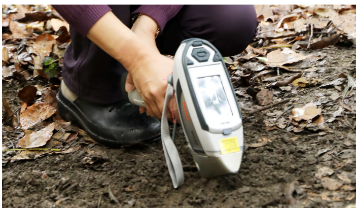
Thermo Scientific portable XRF analyzer for instant analysis of heavy metals along the coast of Hsinchu county.
