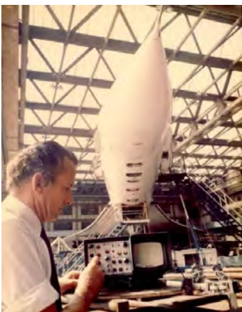
Figure 2: Sonatest UT equipment used for composite assessment on the Concorde program in the UK, late 1960s.
