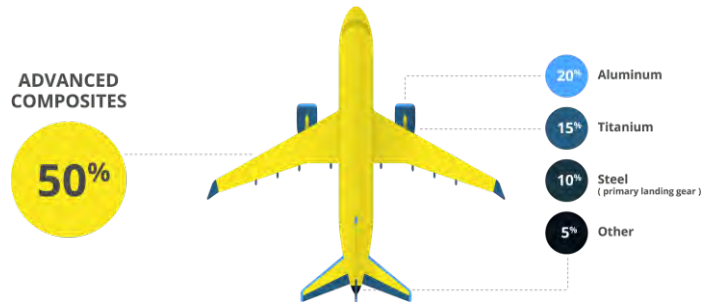
Figure 1: Trend in material composition of the latest aircrafts
