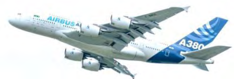
Figure 9: A380 length 73m, wingspan 80m
