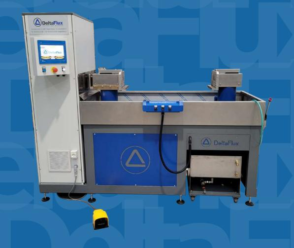
The DeltaFlux MB 50-70-100 FE PBM series is a versatile solution that can be used for testing of pieces with different sizes, weights and shapes. This system is usually used for small to medium part length and weight. Thanks to multidirectional magnetization this system is specially designed for high production requirements.
