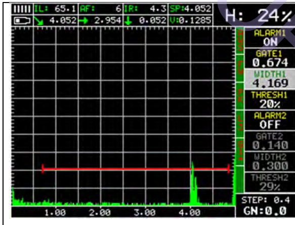
3/64" SDH @ 4" IR (Indication Rating) 4.3
