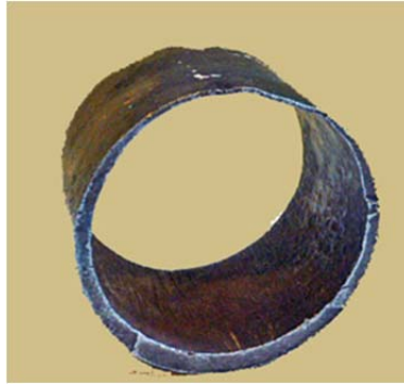
Figure 2 Pipe with severe thinning
