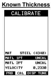
**Note:** Be sure a probe zero has been performed prior to calibration.
