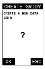
3) Press the ok key to save the **Grid**, or the esc key to cancel the setup and return to the **DATA** menu.
