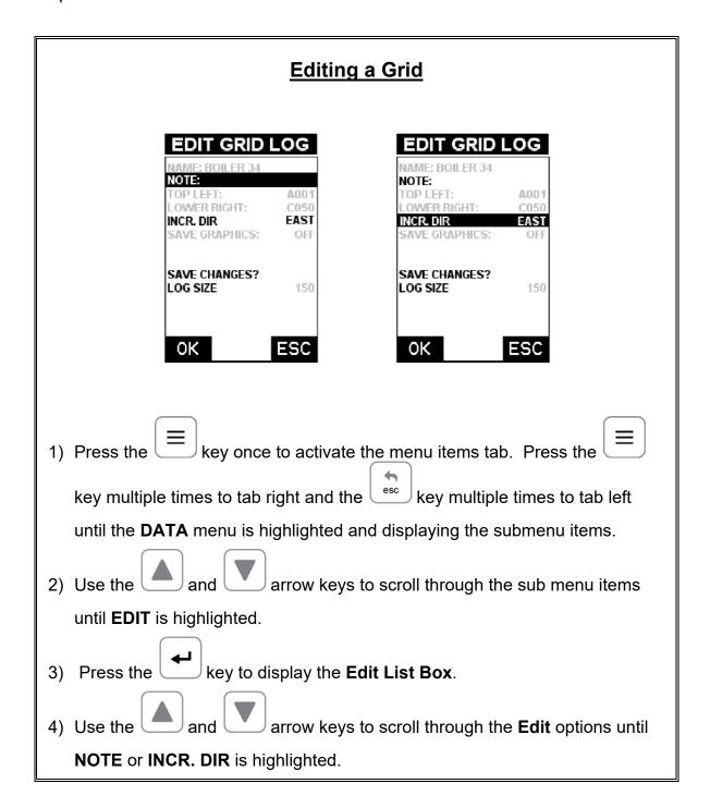
Note: If editing the INCR. DIR, simply use the or arrow keys to scroll NONE, NORTH, EAST, SOUTH, WEST for a Grid, or INC, DEC for a Seq Log. Proceed to step 10.
