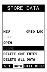
3) Press the key to close the active file. **Note:** Following the key press, the **CLOSE** text will be grayed out indicating the file has been close and is no longer active.
