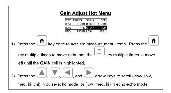
The user can also access and adjust the gain from the tabbed menus however this method is more tedious than making the adjustments using the **Hot Menus**. The procedure using the tabbed menus is outlined below:
