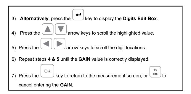
The user can also access and adjust the gain from the tabbed menus. However, this method is more tedious than making the adjustments using the **Hot Menus**. The procedure using the tabbed menus is outlined below:
