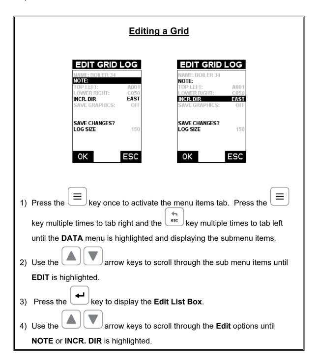
Note: If editing the INCR. DIR, simply use the arrow keys to scroll NONE, NORTH, EAST, SOUTH, WEST for a Grid, or INC, DEC for a Seq Log. Proceed to step 10.
