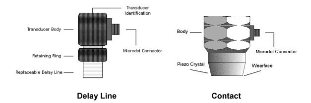
The Transducer is the "business end" of the **PZX1-DL**. It transmits and receives ultrasonic sound waves that the **PZX1-DL** uses to calculate the thickness of the material being measured. The transducer connects to the **PZX1-DL** using a single shielded coaxial cable with microdot connectors.
