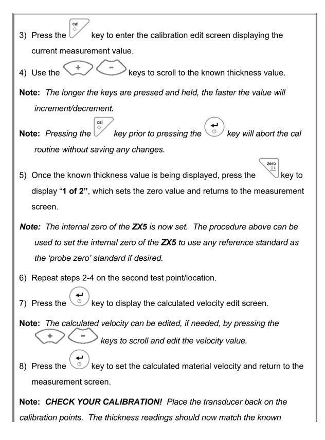
thickness values with minimal error. If the thicknesses are not correct, repeat
