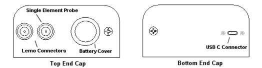
The top end cap is where all connections are made to the **ZX5**. The diagram above shows the layout and description of the connectors:
