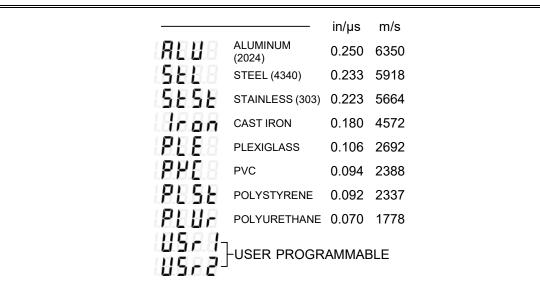
5) When the desired **MATL** setting is displayed, press the key to set the material velocity and return to the measurement screen.
