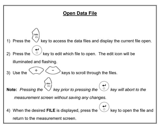
**Note:** The **FILE** and **LOC** (location) will be displayed in lower left portion of the measurement screen.
