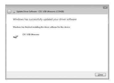
Open device manager again to reference the communications port assigned to the CDC device, it will be displayed to the right of the CDC device. Now that the driver has been successfully installed, a 'keyboard wedge' with serial communications capability can be used to connect to the PZX1 and will capture the measurements to your PC when the ENTER key is pressed:
