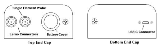
The top & bottom end panels are where all connections are made to the *RX8-DL*. The diagram above shows the layout and description of the connectors:
