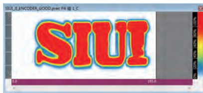
C Scan In-Amplitude, showing echo amplitude
