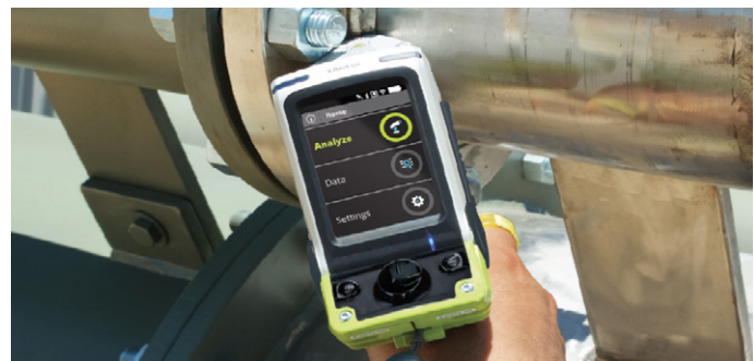
The Niton XL5 Plus analyzer in use, analyzing a tight weld in an oil refinery.
