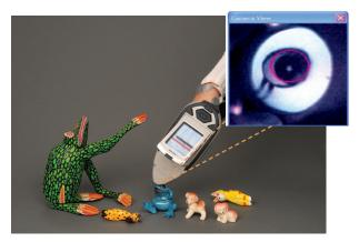
CCD camera and small-spot feature isolates and stores small sample area measurements.
