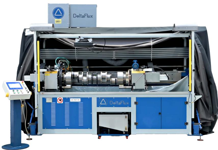
The DeltaFlux Automated Crankshaft Inspection System is a MPI bench designed for production inspection. The system combines automatic pole positioning, coil movement, particle application, part rotation and demagnetization into a one-touch operation, significantly reducing operator involvement and improving inspection consistency.
