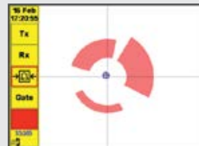
Impedance Plane (XY) Trace with multiple sector gates
