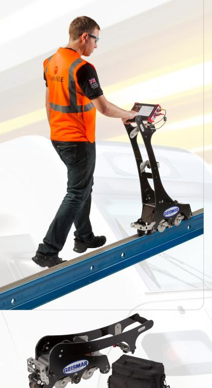
The FILUS EC-1 Trolley is a hand-pushed trolley, specially designed to check a single rail using Eddy current methods.
