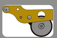
A rotary encoder to provide distance information to the software and synchronise the sample rate with the speed.
