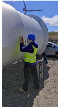
Prototype being used on site for wind turbine blade inspection
