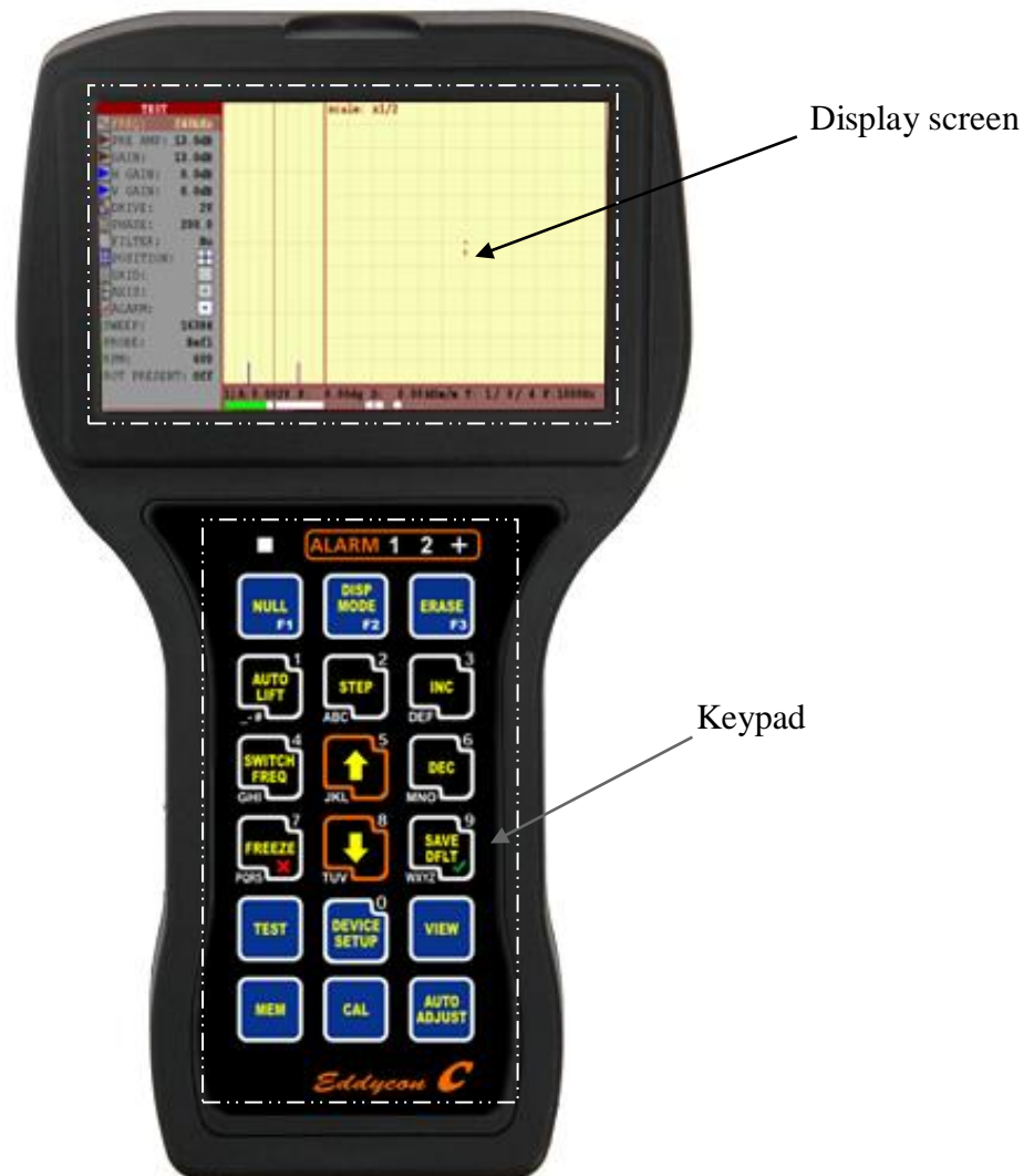
Figure 5 – «Eddycon C» eddy current flaw detector
