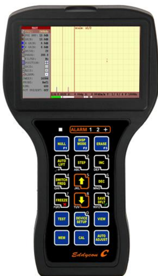
Figure 1 – «Eddycon C» eddy current flaw detector. Front panel
