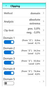
Range limits (time values) are ideally set in such a way that there is exactly one echo to be evaluated in each time period. The time range of the first echo does not have to start at position from Z = 0. The range can also be selected so that possible false echoes are suppressed at the beginning of the time range.
