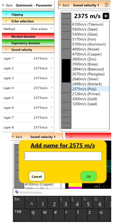
The corresponding configuration window, in this case Sound velocity 1.
