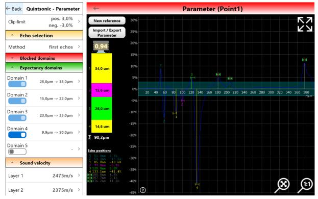
An expectancy domain is completely defined by its lower and upper limits (layer thickness values). In the A-scan, expectancy domains are indicated by horizontal lines in the width of the tolerance band. The assignment to the respective layer is determined by the position in Y-direction and corresponds to the layer thickness column on the left.
