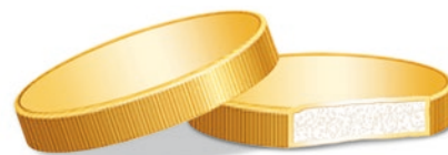
Schematic of counterfeit coins filled with a powdered tungsten alloy and covered with gold
