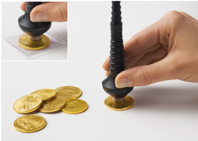
Electrical conductivity measurement on coins – fast and reliable even through plastic covers
