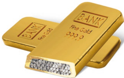
Schematic of counterfeit gold bar with a core of tungsten sticks and gold cover
