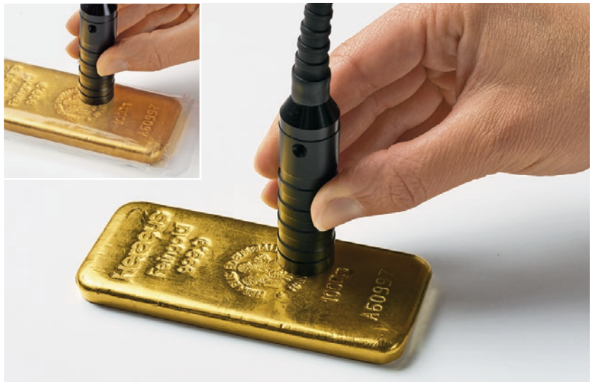
Testing of a fine gold bar – even under a plastic cover
