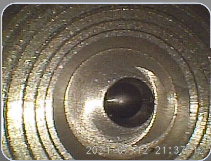
Thread and cross hole inspection in a machined part using a E-Series Video Borescope
