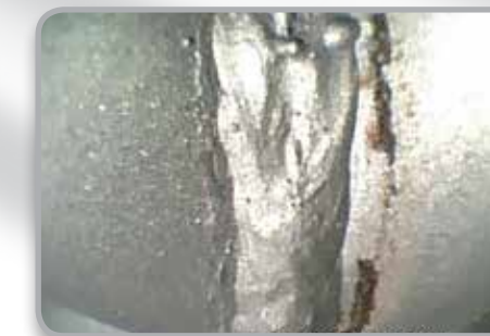
Orbital Weld (Using a 90° Prism Tip)
