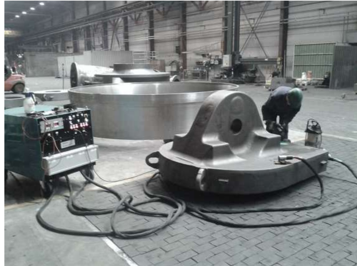
MPI performed with the Multipuls-E3 device on large components with rough surfaces in the foundry of Allard-Europe nv in Turnhout, Belgium
