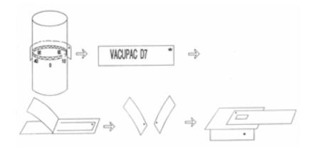
The unpacked film must be turned around in longitudinal axis. This is to make sure that texts of Marking, IQIs and measuring tape can be read correctly.
