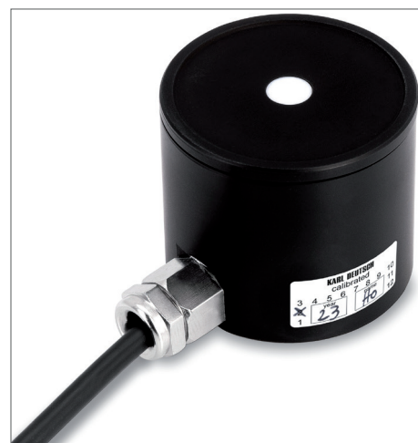
UV and white light probe with translucent diffuser through which the light reaches the measuring unit in the probe
