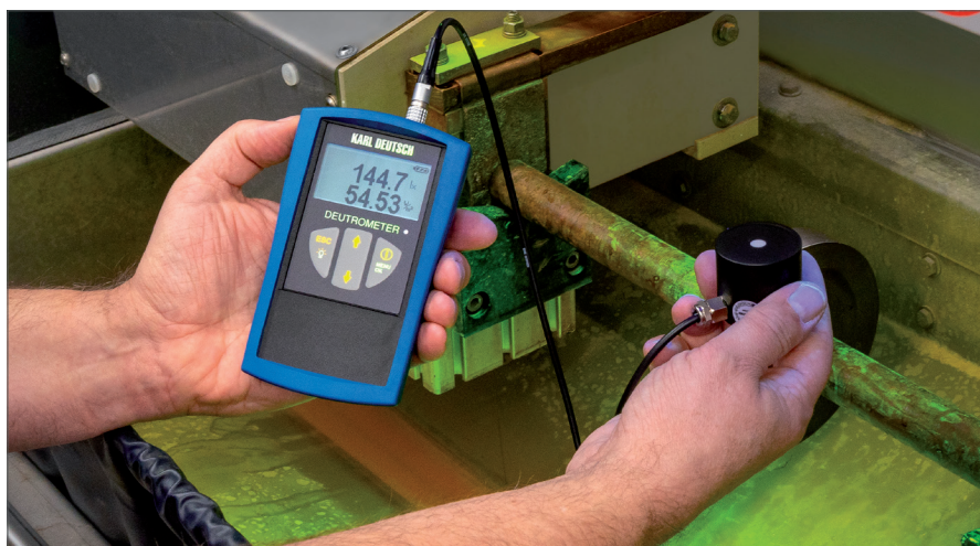
To control the viewing conditions, the DEUTROMETER together with the DEUTROLIGHT probe simultaneously provide the measured values for the residual daylight and the UV intensity
