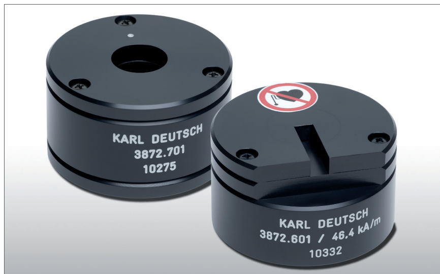
Zero field chamber (left) with field-free inner space and reference magnet with defined field strength are accessories for field strength measurement and used for checking the gauge
