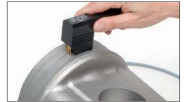
Crack depth measurement of an inclined crack after angle determination
