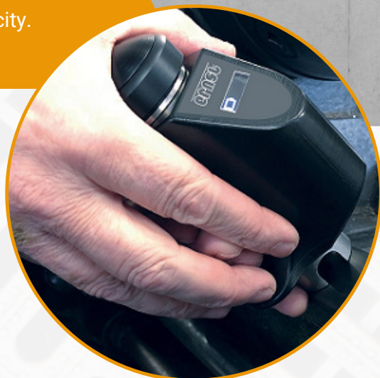
ePortaRock L 5 kgf load capacity
