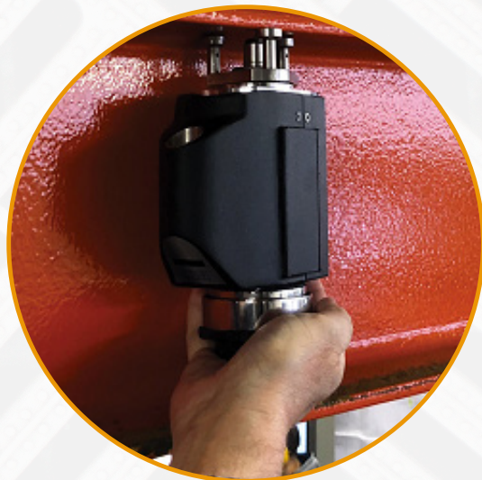
ePortaRock H 100 kgf load capacity
