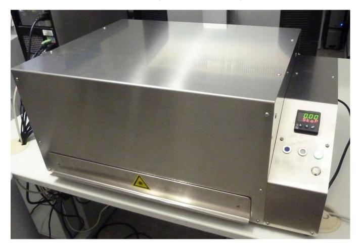
The Koworase X erases burn-in artifacts (i.e. x-ray exposures) from Computed Radiography (CR) phosphor plates with UV radiation.
